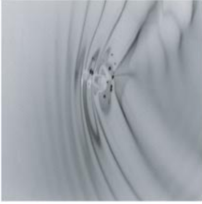
FIG. 22. Image of the capillary-gravity surface waves generated on water by a 3.14-mm-diameter ball.
